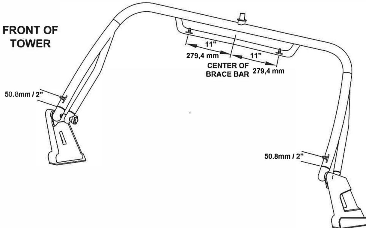
1) MEASURE 2" (50,8 mm) UP FROM WELD ON TOP SIDE FOR CENTER OF MAIN BOW MOUNT. PLACE MOUNT SO IT SWIVELS TOWARDS INSIDE OF BOAT. ATTACH WITH SELF TAPPING SCREWS.
